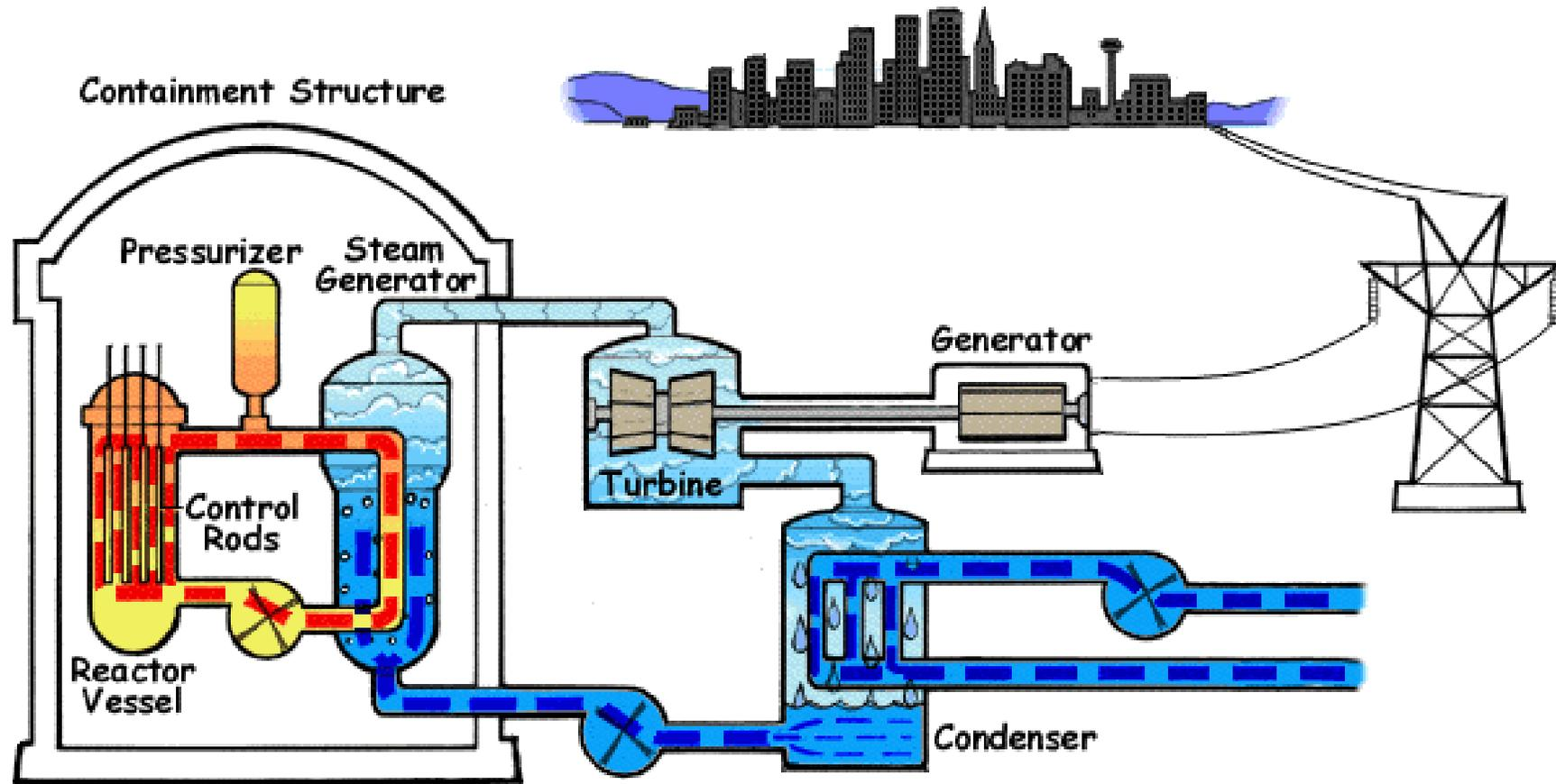
**Pressurized Water Reactor (PWR)**
